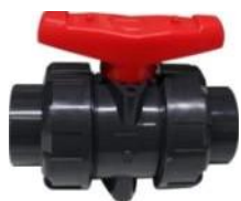
F71 Double Union Ball Valve Size: 1/2"to 4" thread,socket 1/2"-2": 23Spsi Max. 2-1/2-4": 150psi Max.
